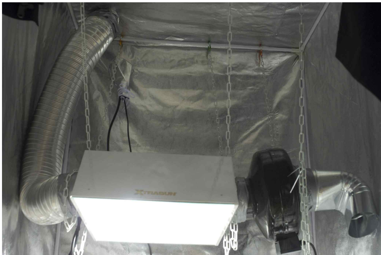
This picture shows the old way I used to mount the duct fan, similar to the new way. That metal piece attached to the duct fan kept falling off only duct taped like it is in this picture, bungee cords fixed that.
