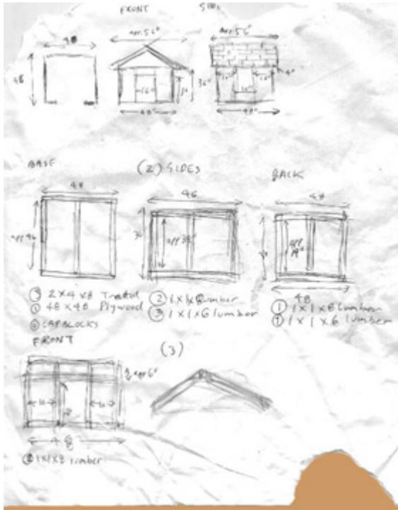
Rough plans for the dog house. Note that beneath each small drawing I have made a list of materials to be used in that section. Please note the semi-circular chunk taken out of the lower right hand corner. I swear to you that my dog Mavis started eating the plan when I turned my back for a minute. Oddly enough, I was ten years out of college before my dog actually did (try to) eat my homework. Oh, well.
