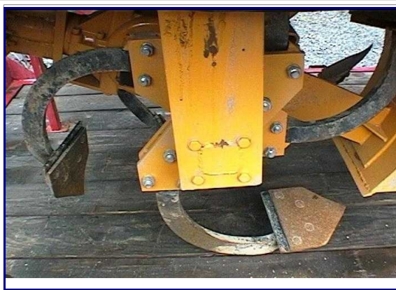
Close-up display of shovels on an Imants spader, a rotating-type spading machine.
