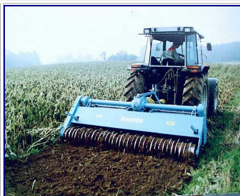
Imants spading machine in the field; working down crop residues in one pass.
