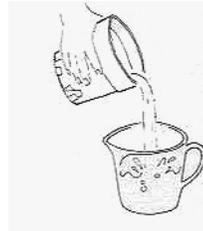
Figure 3. Determination of total volume of pot.
