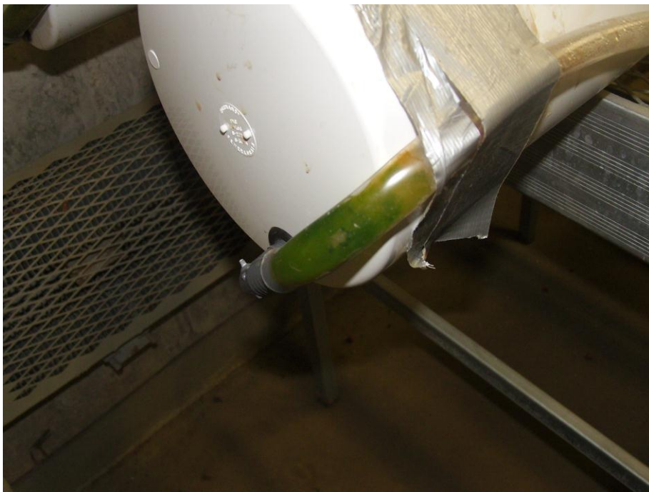
Figure 8. Algae growing in the outlet hose of a tube A.
